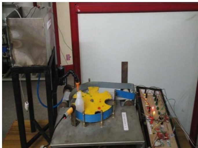
Figure 5 Fabricated Prototype automated carousel bottling system model
